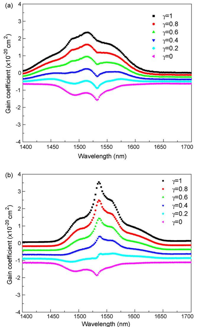
Fig. 3. Gain coefficient in the eye-safe range of  $Er^{3+}$  in (a) the MBBA system and (b) the BBBM system.
